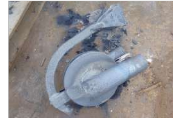
Flash-less castings, minimal grinding
