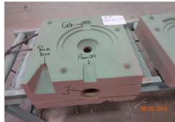
Conventional no-bake molding Printed Sand $0.08-$0.15/cu. In.
